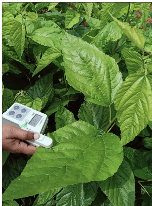
Figure 1: Recording of chlorophylls using SPAD meter
